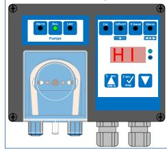
The controller is in the mode hand dosing (HI)
