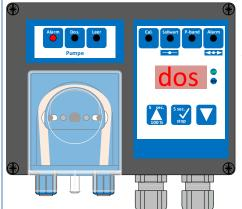
If the target value plus a hysteresis (0.1 pH or 10 mV) is not reached within the adjusted time (Alarm doS), the dosing is deactivated. The display changes between the real value and **Dos**. The dosing time limitation finishes internally, the time already finished is not visible.
