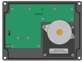
To change the measurement dimension pH  $\leftarrow \rightarrow$  mV the casing must be opened. At the left side of the console there is a jumper (short-circuit bridge).
