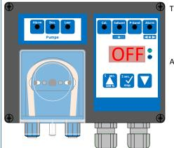
The controller is in the mode manual STOP (OFF)
